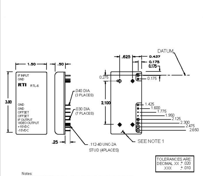
1. This surface should be in direct contact with the mounting surface.
